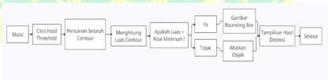
Gambar 3.11. Diagram gambar Alir Proses Contour Detection
