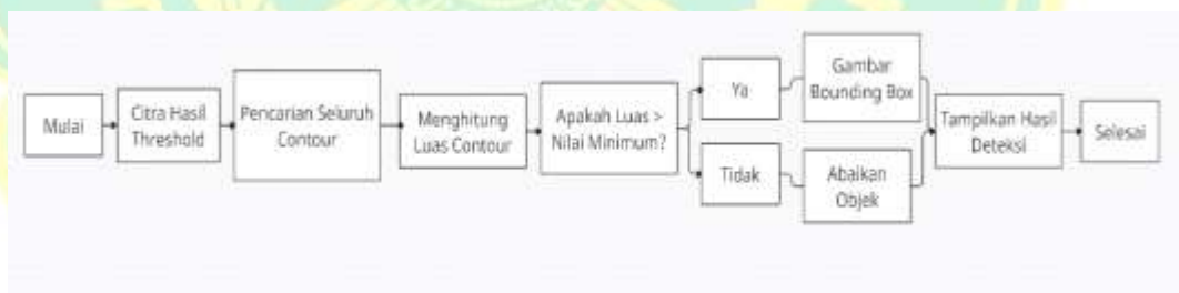
Gambar 3.11. Diagram gambar Alir Proses Contour Detection
